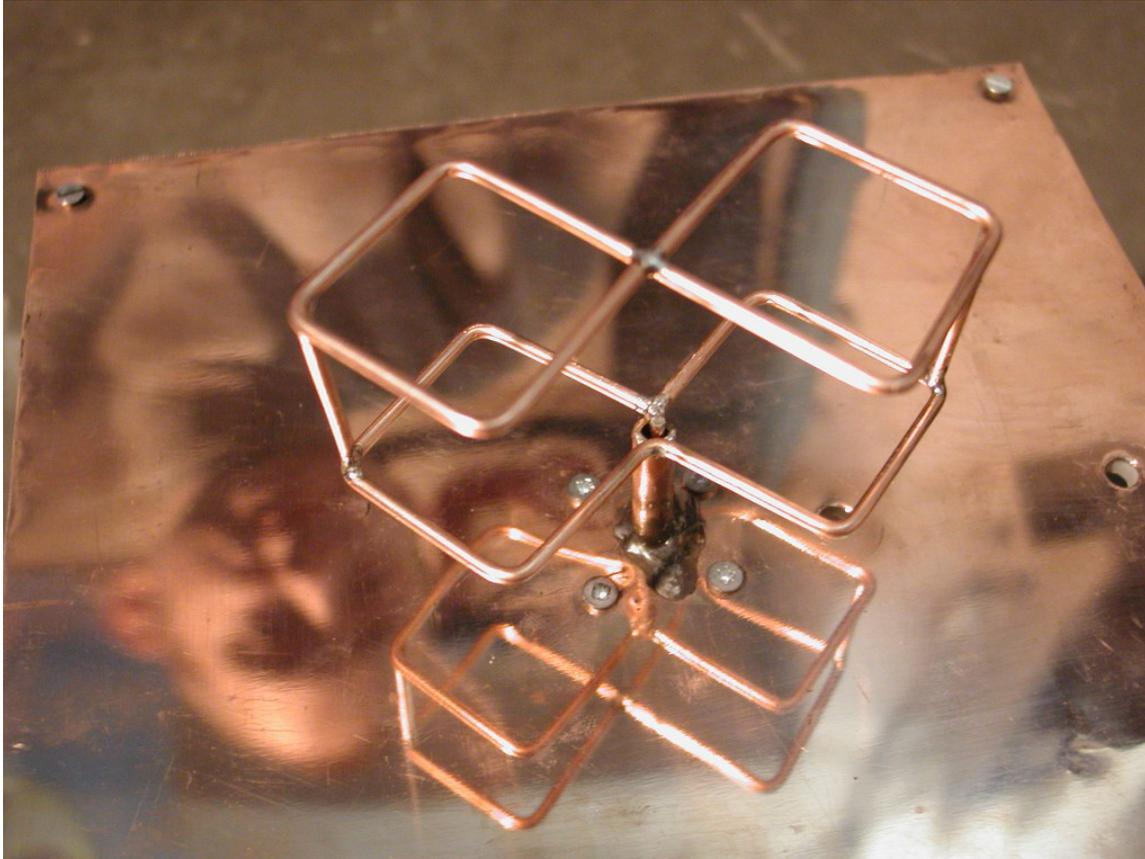
*Fig. 21. Feeding of 2 el. bi-quad feed antenna*
