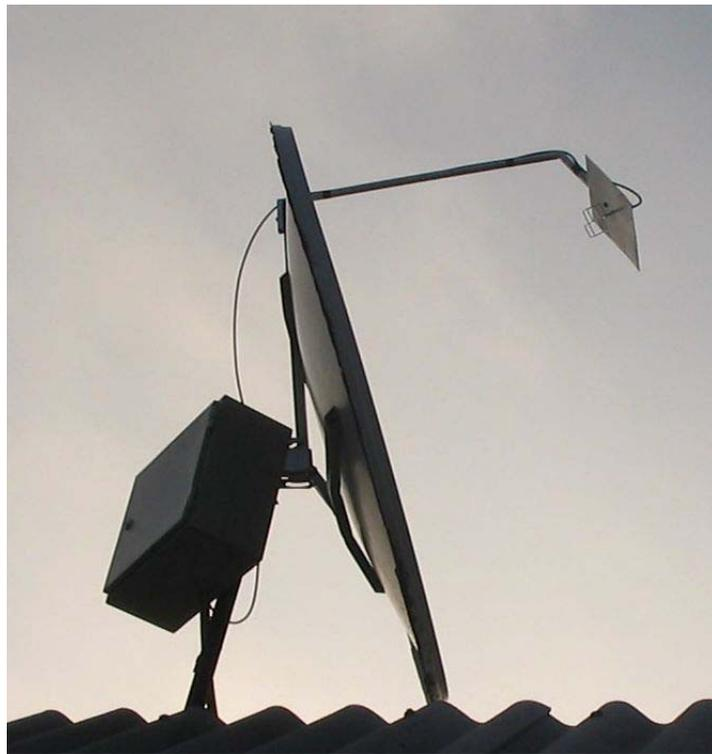
*Fig. 24. Offset dish with 2 el. bi-quad feed antenna*
