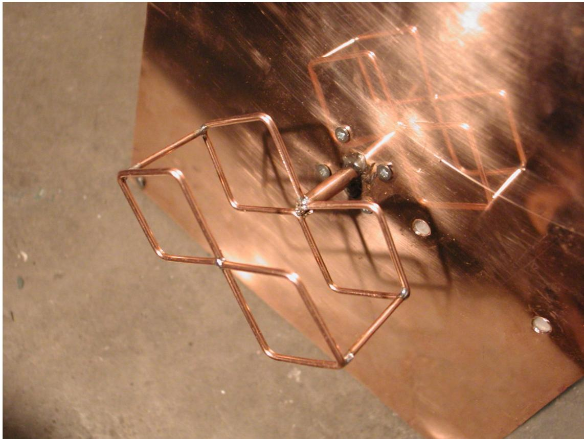
*Fig. 20. Outlook of built 2 el. bi-quad feed antenna*
