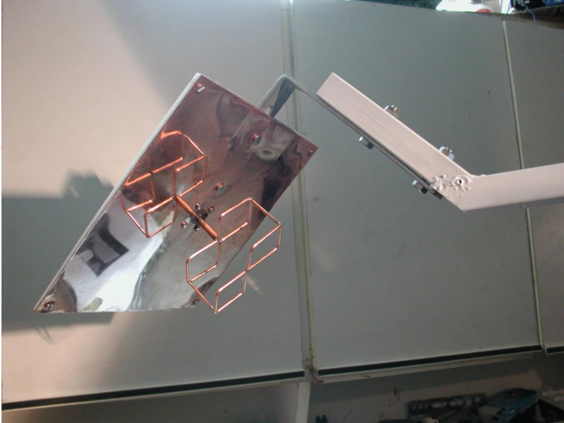
*Fig. 23. Two-elements bi-quad feed antenna on its carrier*
