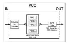
Using PCQ is very simple; however there are a number of things you will need to understand. There are two limits to your PCQ queues, a max-limit which shows the overall queue bandwidth, and a pcq-rate. The pcq-rate is the rate to give the individual sub-queues. If you leave that, the pcq-rate, as zero, there will be no individual queue limit. This will allow us to evenly distribute the max-limit of the PCQ queue regardless of the number of sub-streams.
