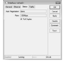
In the Ethernet status window, you will see the current status of your Ethernet port. In this example, we have performed auto-negotiation. We have a link rate of 100Mbps, and are running Full Duplex.
