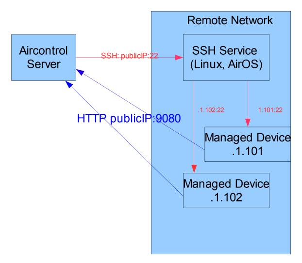
AirControl uses SSH port forwarding ("tunneling") through the SSH host/gateway for all operation that require access via SSH to device (connect, firmware upgrade etc.). Note that access to the AirOS web interface is not supported through this mechanism, this is only for AirControl operation.
