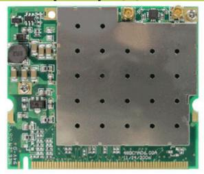
CM10-H (MMCX) is a high power 600mW(28dBm) IEEE802.11a/b/g 108Mbps wifi mini-PCI module with two MMCX RF connectors designed specifically for integration in reliability/performance-critical applications. High power design with advanced **SuperAG** feature, CM10-H (MMCX) is ideal for embedding into super-range and high-speed applications such as outdoor point to point or building to building wireless Access Point/Bridge connections.
